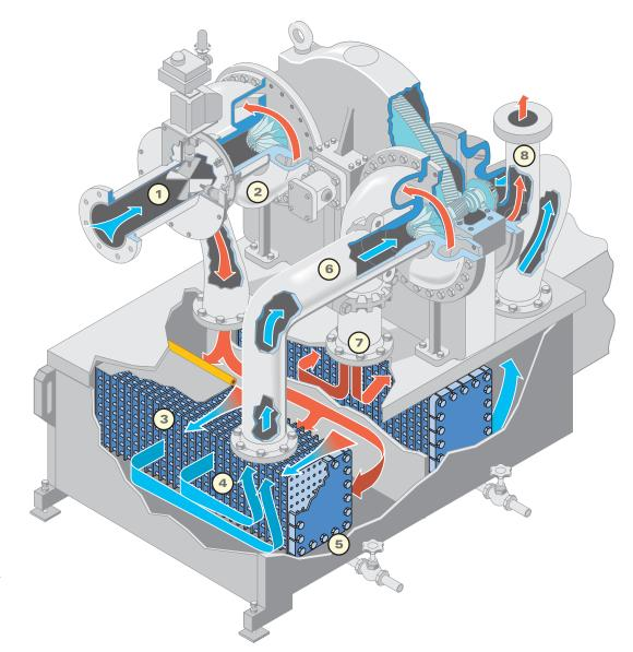
6 The air exits the intercooler and flows into the inlet duct for the second stage. In the second stage the compression process is repeated with an impeller, diffuser, and a scroll casing. **7** The air discharges from the compressor volute and enters the second stage intercooler. The intercooling process is identical to that in the first stage.
